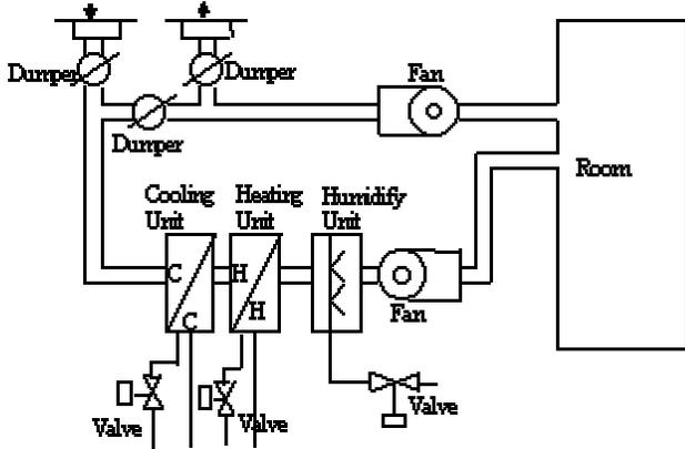
Fig. 2 Composition of the air-conditioning system
